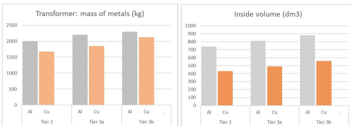
The mass of metals increases with the efficiency level, for a given conductor material. However, there are important material saving opportunities when shifting from aluminium to copper designs (about 20% reduction in total weight for Tier 2 efficiency level). The same shift also leads to a more compact unit, with size reductions in the range of 40%.
