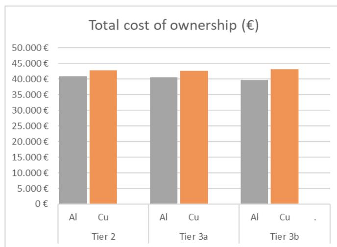
The graph above shows how the total cost of ownership remains relatively flat regardless of the efficiency level and the conductor material selected.
