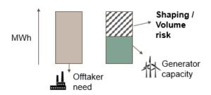
**Volume risk** is the risk that the RES generator does not produce the volume of electricity predicted in long-term modelling. **Shaping / profiling risk** is the risk related to the difference in the stable demand profile of an industry offtaker and the variable supply profile of a RES generator: even if overall generation volume is as expected, the hour-to-hour generation volume of the RES generator is variable and will therefore not always match the demand of the offtaker.
