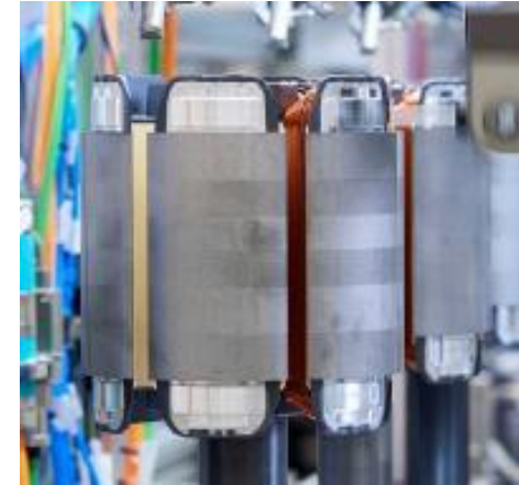
Manufacturing images of BMW's rotor for the new 5 th generation electric drivetrain, suggesting a WRSM configuration. Source: BMW Group
