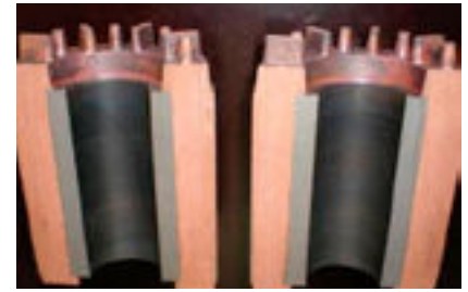
Cross-section Through Rotor Bars and End Ring of Die Cast Copper Rotor
