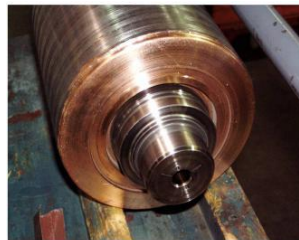
Figure 14 - Copper die cast rotor for the traction motor application.
