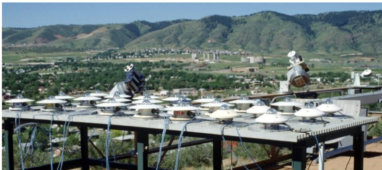
Figure 2 – Irradiance measurement instruments. Rotating shadowband radiometer (upper right). Thermopile pyranometers being calibrated at NREL (lower left).
