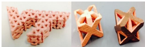
Fig. 4: Cellular hollow Cu structures fabricated using the binder jetting AM process [44].
