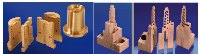
Fig. 2: Tool inserts with internal cooling structures made from Hovadur K220 by SLM [39,40].
