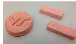
Fig. 8: Sintered copper part samples (AcuPowder 153A copper powder sintered in pure hydrogen at 1000 °C for 8 hours) [47].
