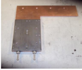
Fig. 15: Multi-metal heat exchanger. Fabrisonic's process can print multiple metals together without causing metallurgical problems. In this structure the high heat areas are made of copper and the rest of the structure is made of aluminum to reduce weight [56].
