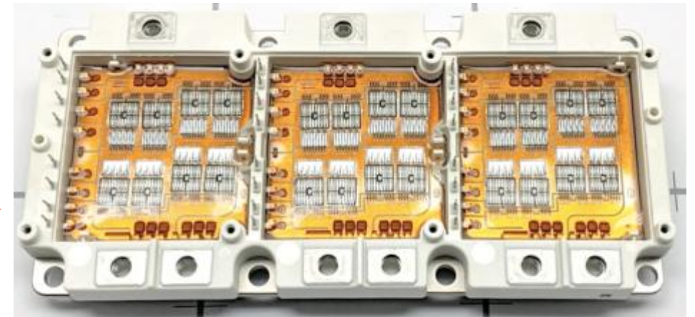
Open view of standard Si IGBT power modules from Infineon. Source: Munro & Associates
